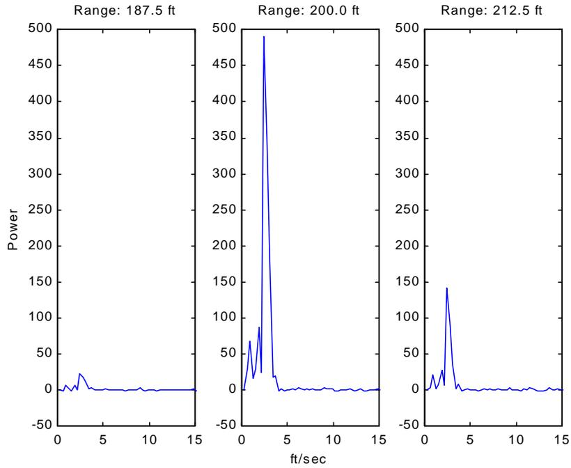
**Figure 11.** Human target walking towards radar at 200 feet.
