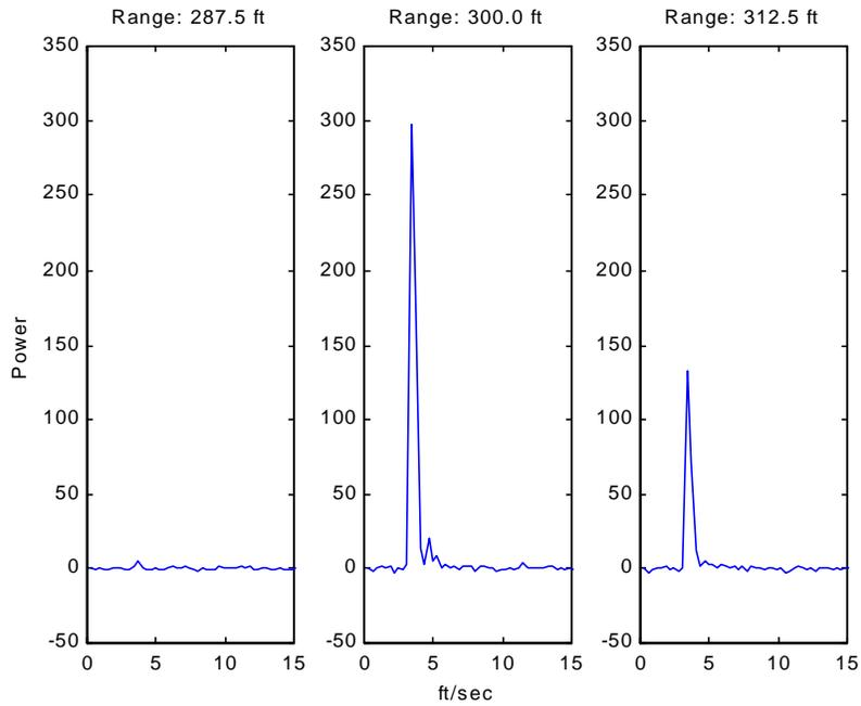
**Figure 12.** Human target walking towards radar at 300 feet.
