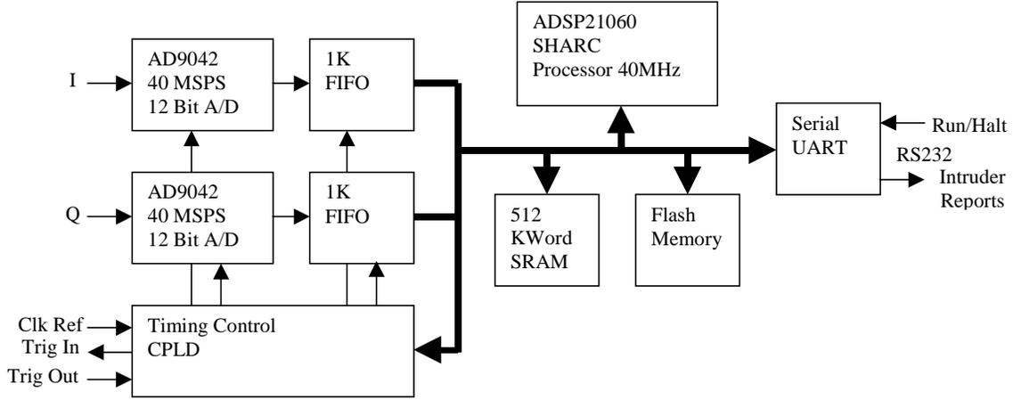
**Figure 9.** Block Diagram of radar processing electronics.
