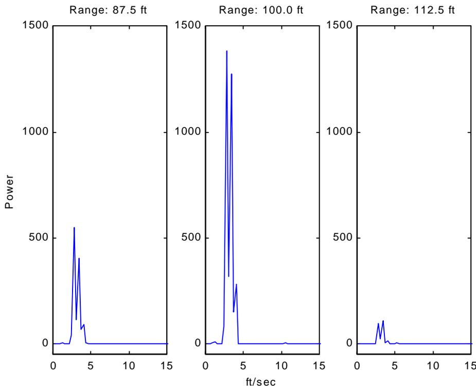
**Figure 10.** Human target walking towards radar at 100 feet.
