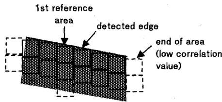
Figure 14. parallelogram area detection using adjacent correlation operation
