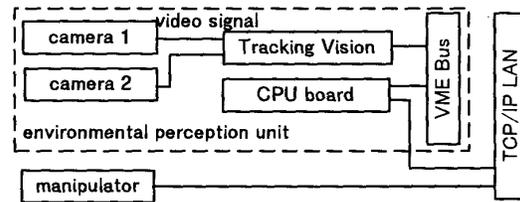
Figure 21. system configuration of the environmental perception unit
