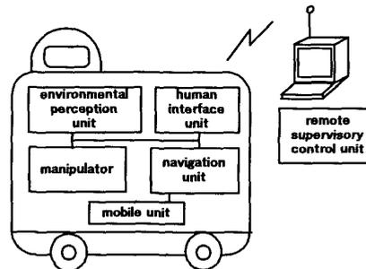
Figure 2. The components of the robot
