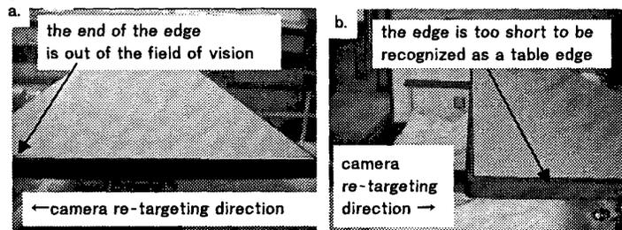
Figure 18. examples of failed camera targeting
