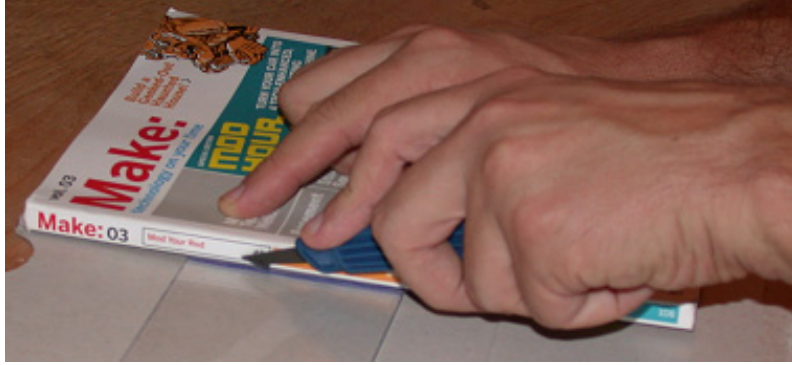
Figure 8. Scoring an acrylic sheet with a cutting tool
